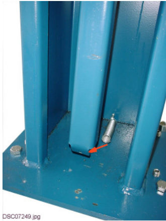
Pic 6: Hang up the spring into the ratchet-strip
