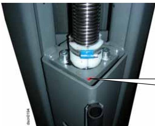
pic 16: the carrying-nut wear pin marked with red safety colour
