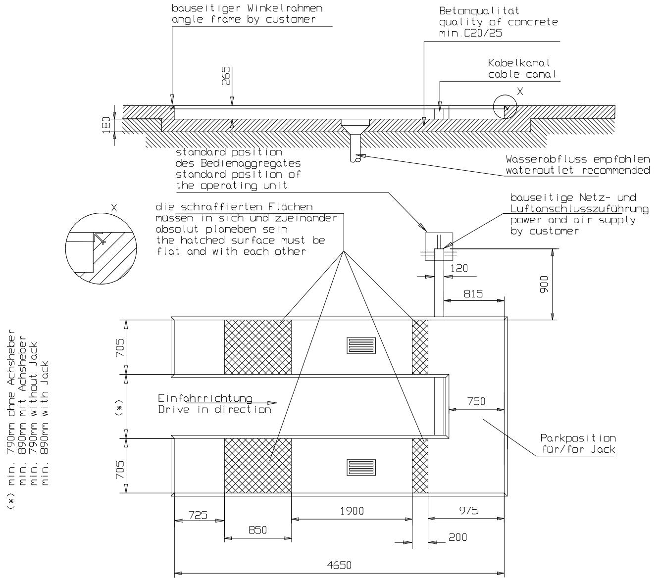
Valid for standard inground version of the lift with drive-on ramp at each side of the platform.
