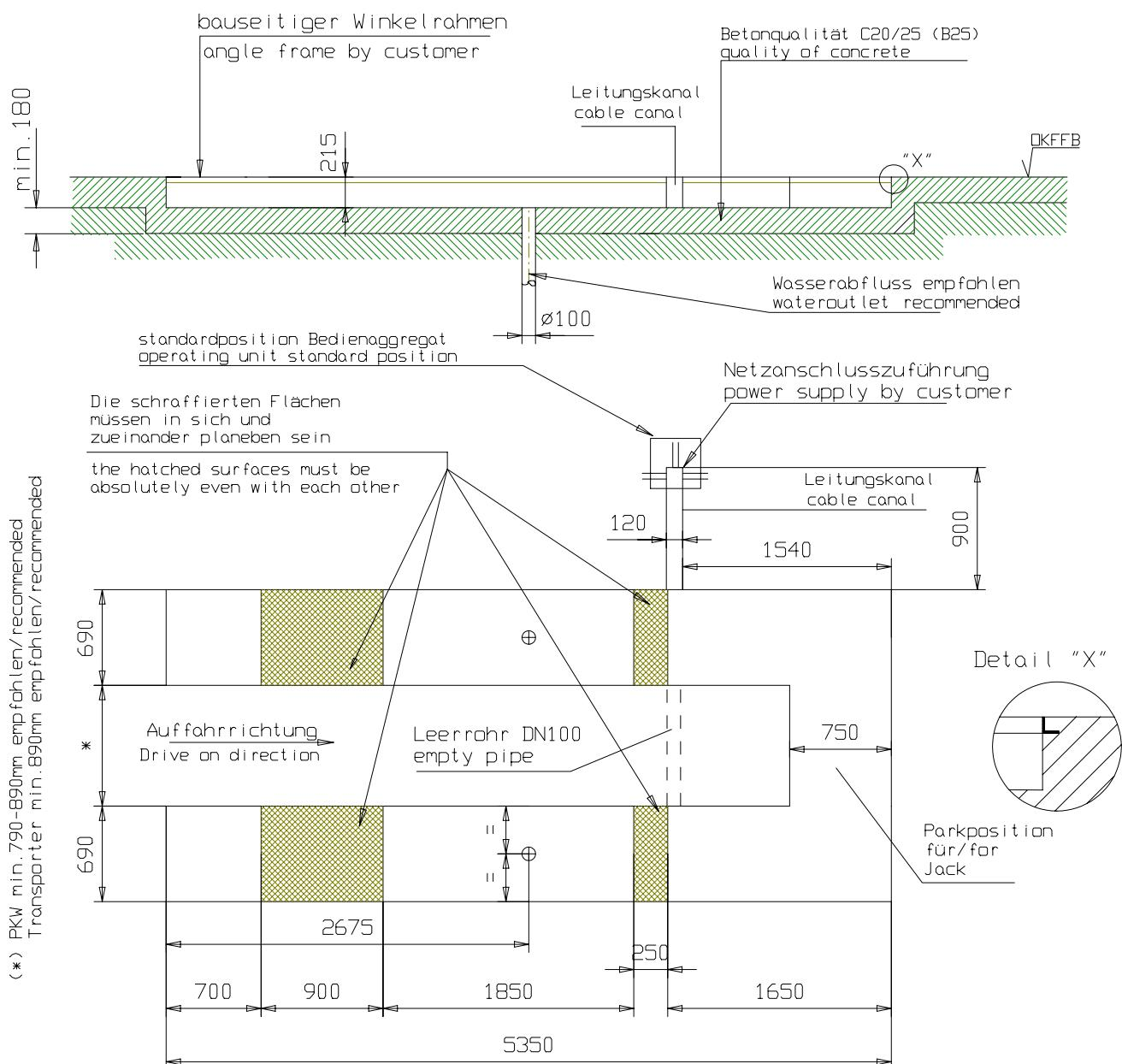
Valid for the standard inground version of the lift with drive-on ramp at each side of the platform. Instead of the cable duct a empty pipe with 150mm diameter can be used to lead the hoses and cables to the operating unit. If desired the position of the power unit can be changed. If necessary adopt the supply lines.
