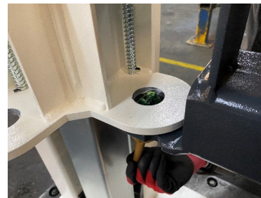
Grease the lower aperture
