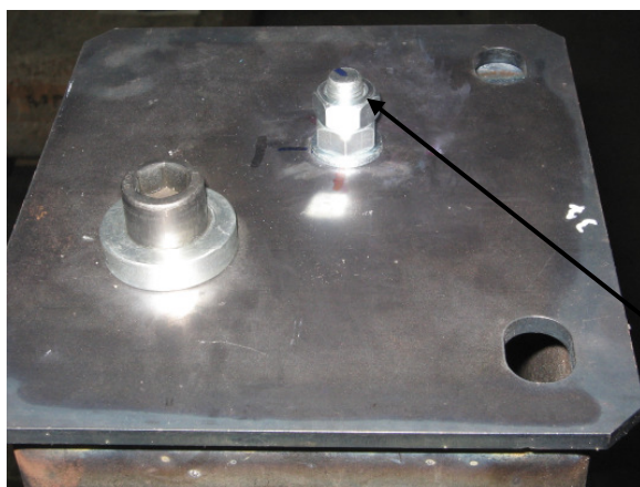
pic.3 counter-locking of the rope on top of column with 2 hex-nuts M12 DIN934 (see example for one Column)
