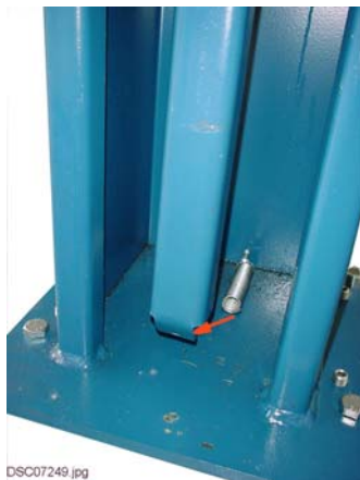
pic 6: Hang the spring into the ratchet-strip
