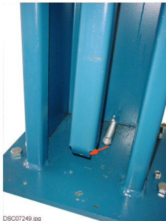
pic 6: Hang the spring into the ratchet-strip
