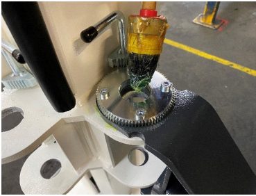
Grease upper aperture
