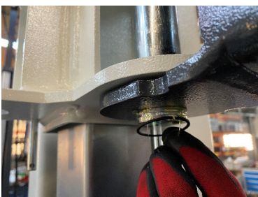
Fit lower circlip to pin
