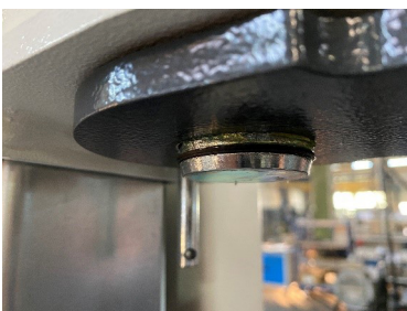
Lower securing pin of the support arm pin
