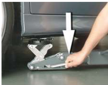
Figure 2: If required, place the carrier plate by pushing the lever at the fixture points.
